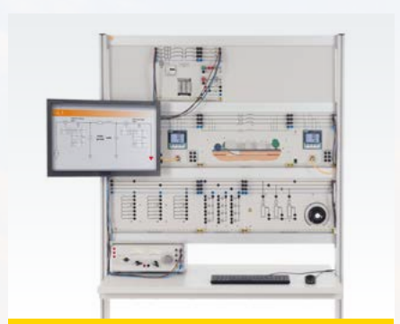
EUL 5 - Investigations on three-phase cables
