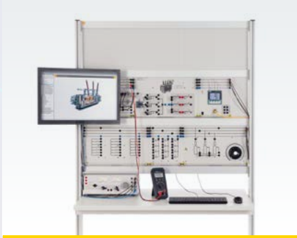
EUT – Investigating Transformers
