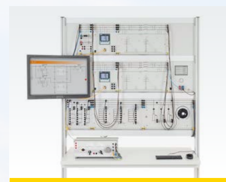
EUL 1 - Investigations on three-phase transmission lines
